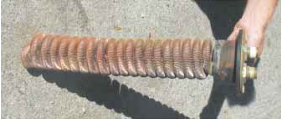
An internal, integrated (and removable), fin-type heat exchanger.
