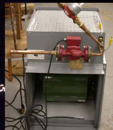
Fan Coil (Boiler)
