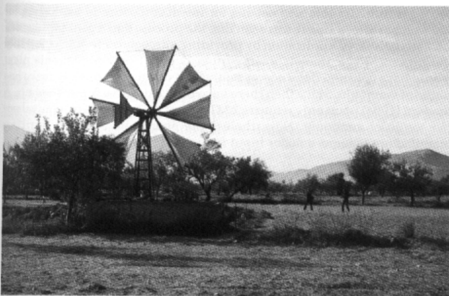
Figure 3.3 A traditional irrigation windmill at work in Crete (photo Bob Everett)
