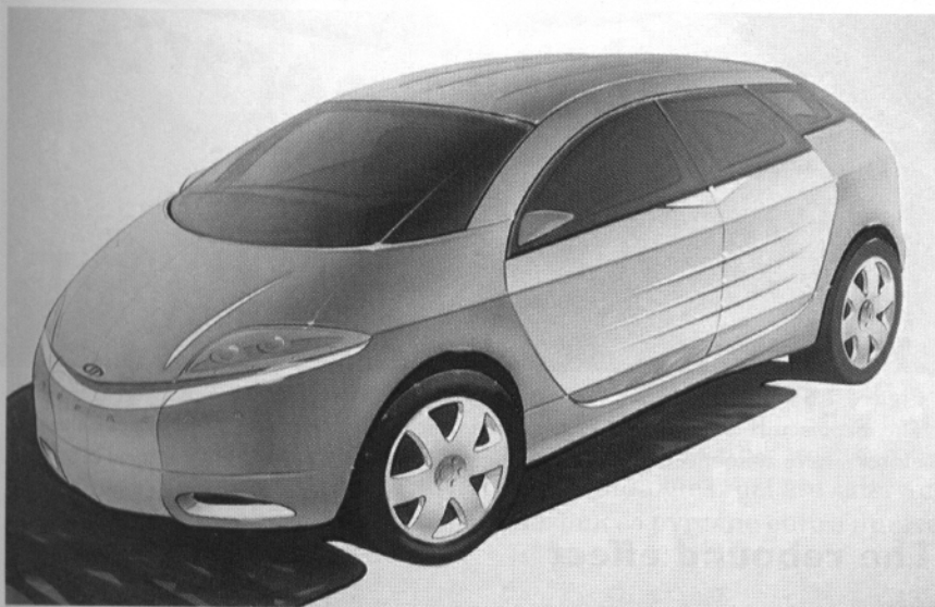
Figure 1.52 The 'Hypercar', designed by engineers at the Rocky Mountain Institute, Colorado, USA, would be streamlined and made of strong but ultra-light, composite materials
