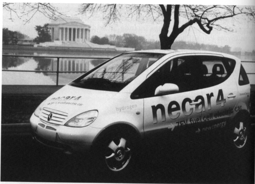
Figure 1.53 This Mercedes A-Class car is powered by a fuel cell running on hydrogen. The manufacturers, Daimler-Chrysler, and other car-makers such as Ford and General Motors, have announced plans to introduce similar cars on the market around 2004
