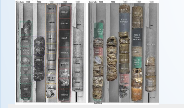
On the left, the ice core tubes catalog by Fountain, and on the right, the reconstruction from samples cut in 1972 made by Andrew Christ (Fountain et al., 1981; Bierman et al., submitted.)
