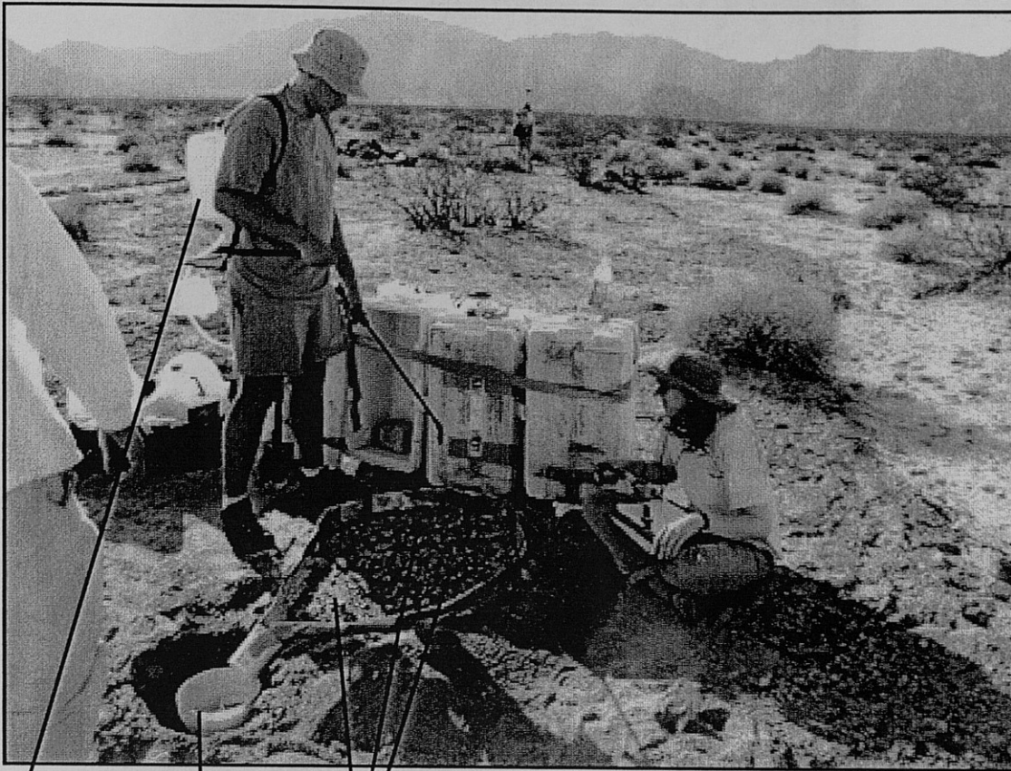
Pump Sprayer Outlet Bucket Rain Gauges
