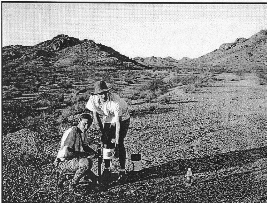
Figure 1.5 - Rain Gauges were installed at three of the four sites. All gauges were installed vertically on a metal pole. East Range Road did not receive a rain gauge. Data from the rain gauges were downloaded by laptop computer.
