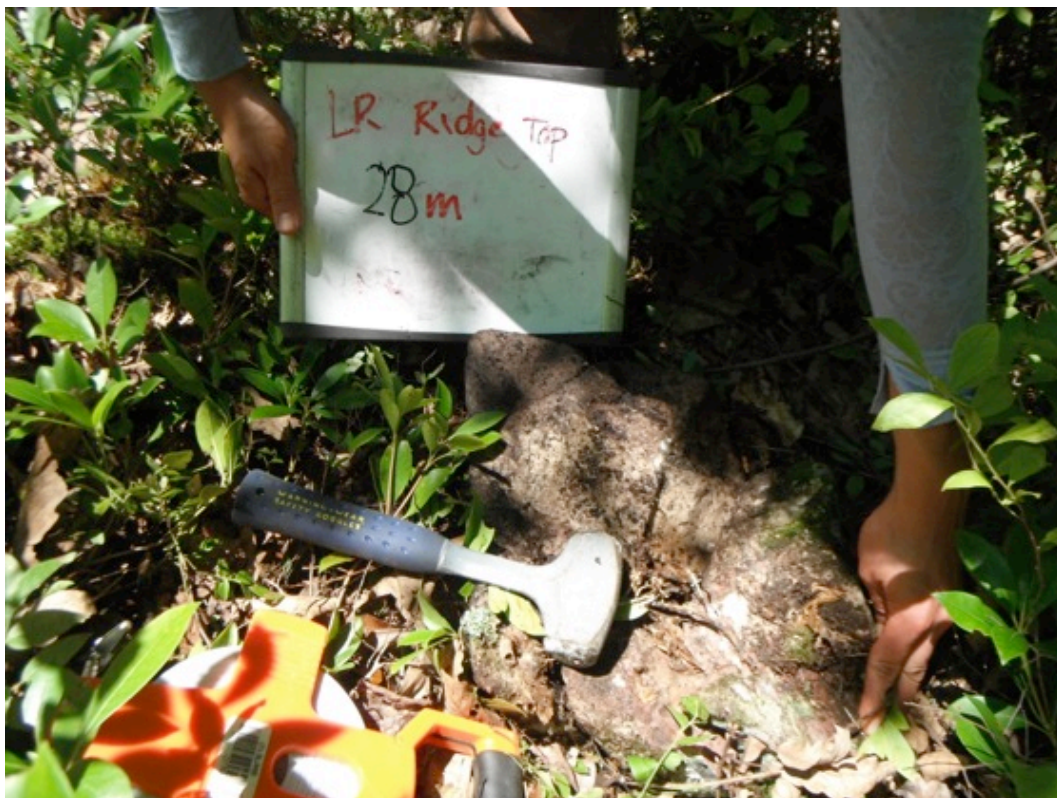
Figure 4. Typical Tuscarora quartzite boulder sampled on Leading Ridge at Garner Run site.
