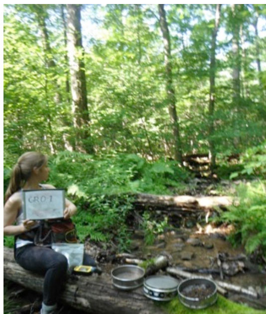
Figure 5. Sampling stream sediments at Garner Run. Sediments were sieved to the 850-250 \mu\text{m} fraction in the field. The streambed is shallow, \sim 3 m wide, and covered in quartz sand and angular quartzite cobbles.
