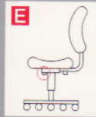
*Tilt tension Controls rate and ease of recline
