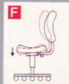
*Forward tilt lever Provides tilting forward.
