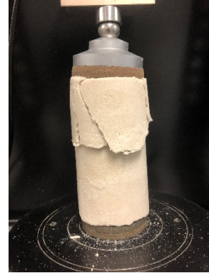
Figure 2. Unconfined compressive strength failed specimen (2.5% moisture content) of frozen regolith simulant (F-75 sand).
