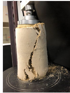
Figure 4. Unconfined compressive strength failed specimen (10% moisture content) of frozen regolith simulant (GRC-3).
