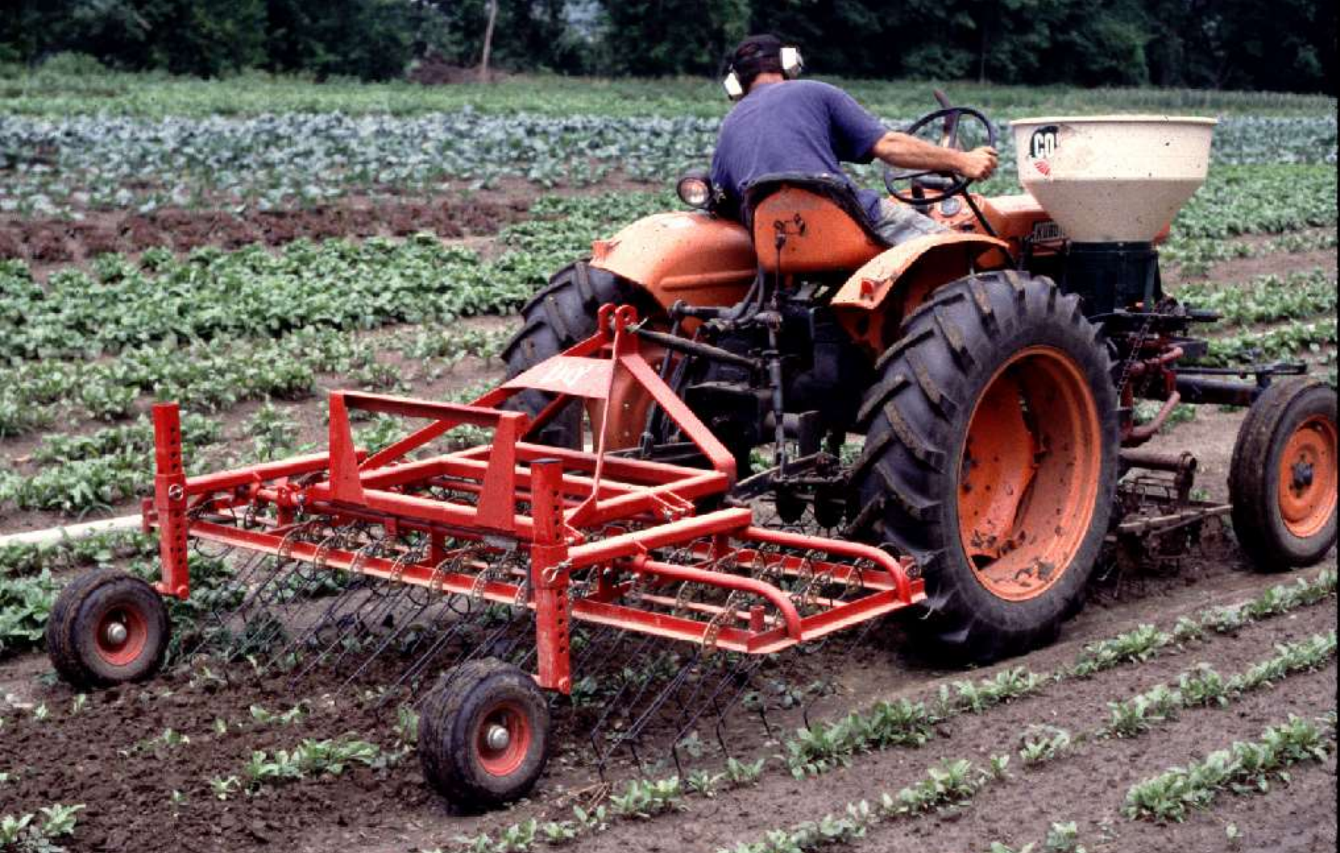
tine weeder with gauge wheels plus belly-mounted baskets
