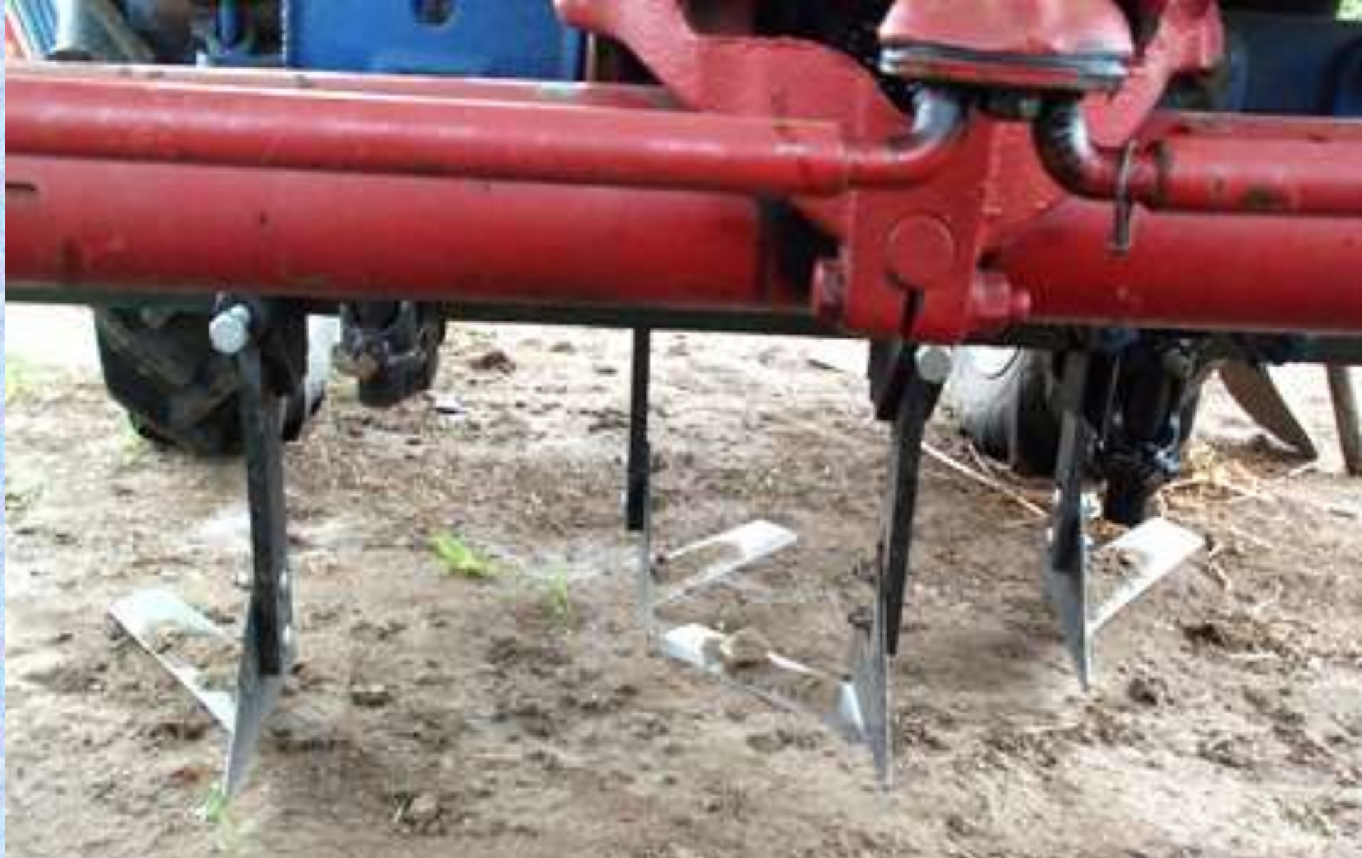
side-knives to reduce depth and soil movement vs. shovels
