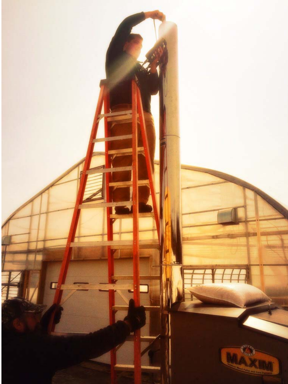
Figure 17 - Testing basic emissions and boiler thermal efficiency at Jericho Settlers Farm (Jericho).
