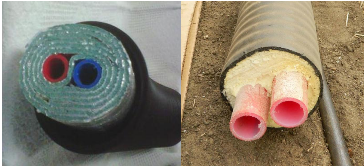
Figure 27 –A less expensive underground insulated PEX tubing option (left) is wrapped in foiled bubble wrap and has space between the insulation on the pipe as well as the outer wall. Cost is approximately $7.00/ft. The solid EPS insulated PEX tube (right) is more expensive at $11.00/ft but has demonstrated reduced heat loss and pipe to pipe heat transfer. Water infiltration is a concern on the foil wrapped version on the left due to the open area that exists.
