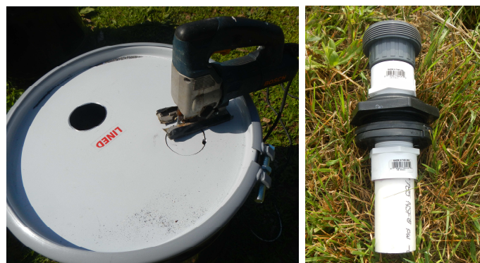
Figure 2. Cutting hole in barrel lid (left) and outlet bulk-head fitting assembly (right).
