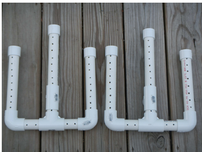
Figure 3. Diffusers constructed by drilling holes in PVC.
