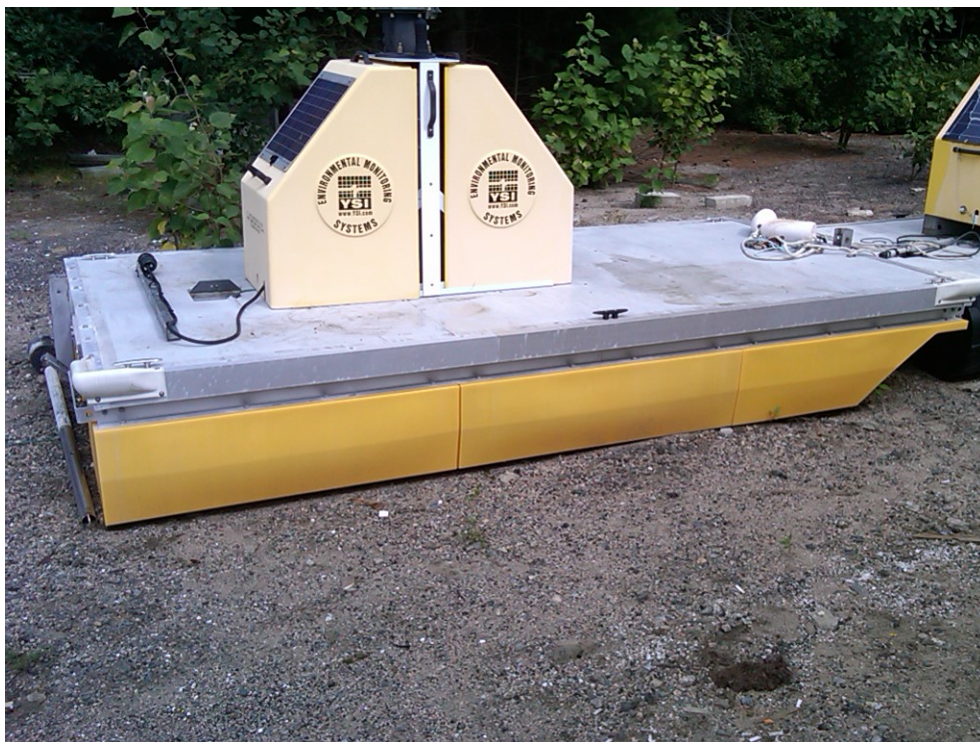
Figure 1. Vertical Profiling Pontoon system from YSI. The winch housing is in the center of the deck. This unit has been completely refurbished for deployment in 2012.
