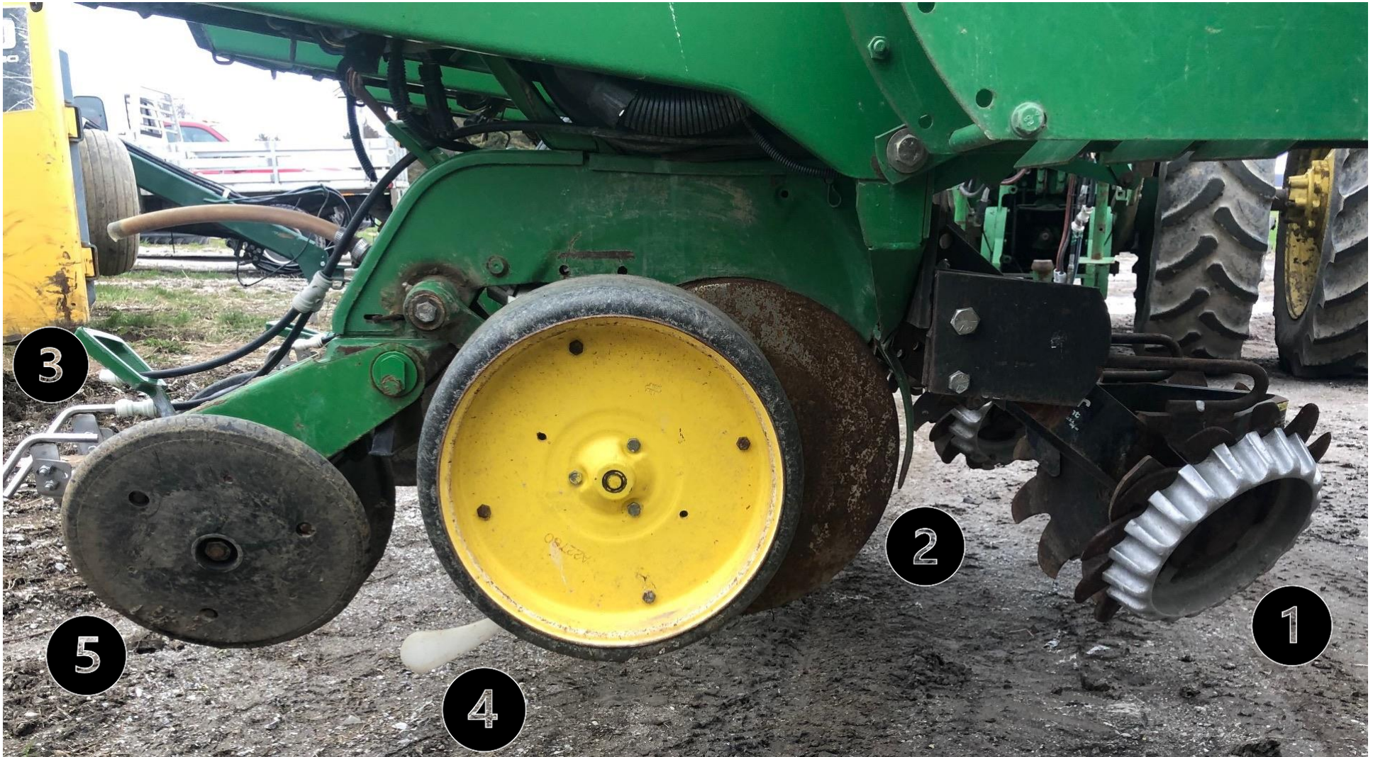
Image 8. Parts of a no-till corn planter row unit.
