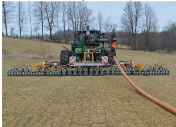
Image 3. Manure injectors for use in no-till cropping systems
