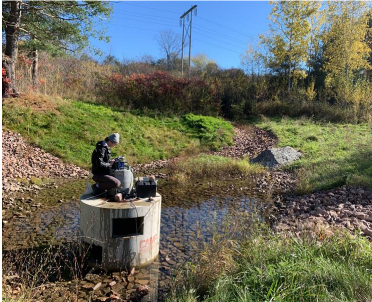
Figure 9. A field technician programming the ISCO.
