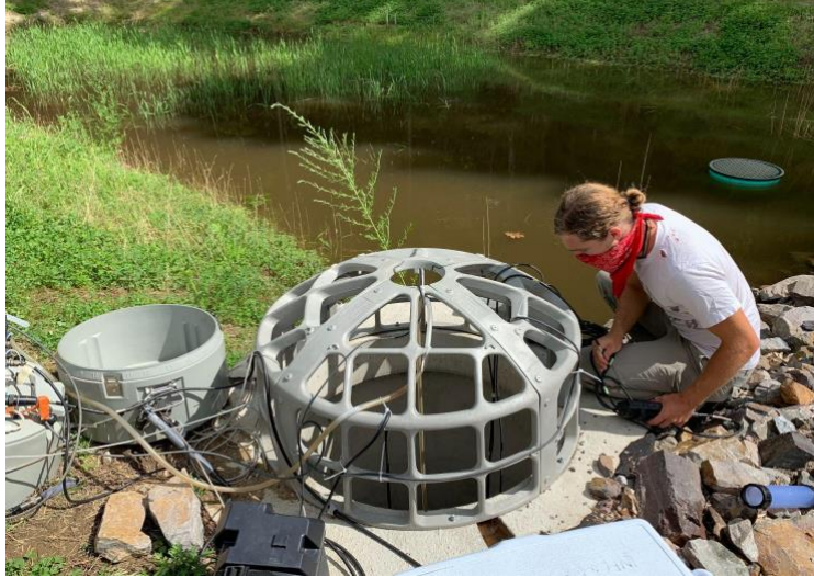
Figure 12. A field technician collecting water quality readings using the YSI multiparameter probe at the outlet of the Kennedy Drive wetland.
