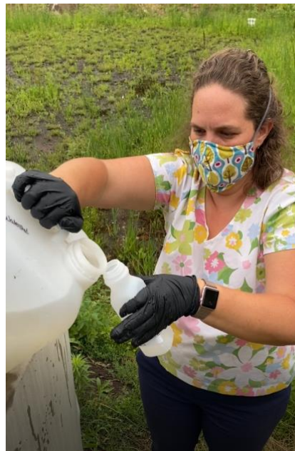
Figure 11. A field technician subsampling the composite water sample collected by an ISCO autosampler.
