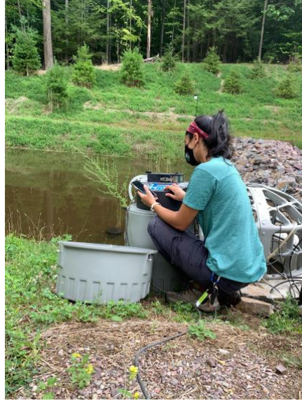
Figure 10. A field technician collecting flow rate data from the ISCO autosampler.
