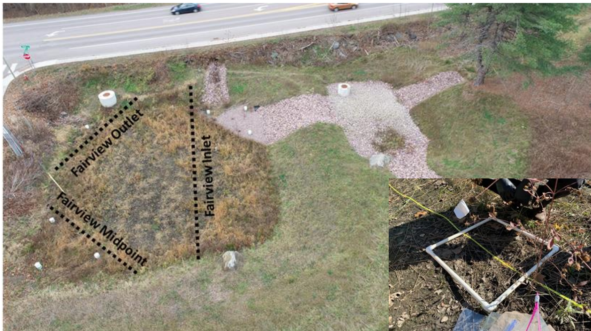
Figure 14. Vegetation and soil sampling cross sections at the Fairview Drive wetland and an example of 0.25m 2 quadrat along cross section.
