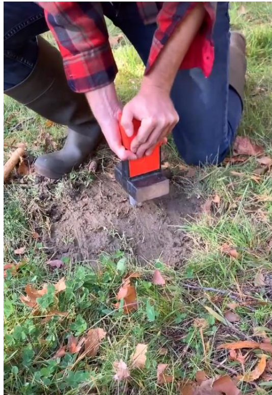
Figure 17. A field technician providing a tutorial on soil core sampling at an adjacent upland site using a 60 mL plastic syringe and a wooden weight.
