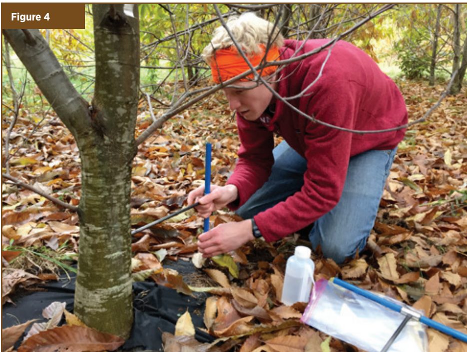
Collecting a tree core using an increment borer.
