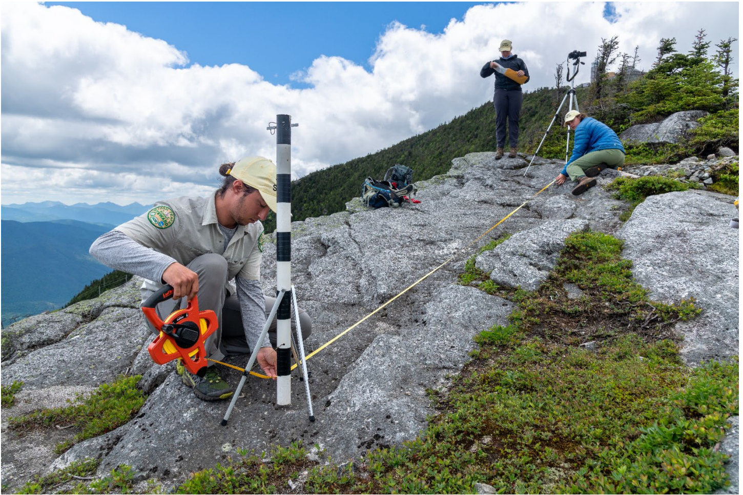
Figure 1. Photopoint Monitoring Field Tech and summit stewards setting up the meter stick at an established photopoint.
