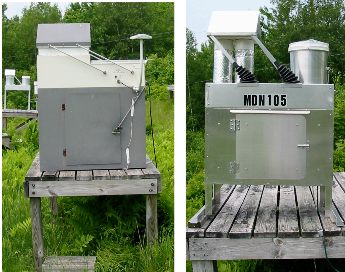
Figure 1. The University of Michigan MICB (left) and Mercury Deposition Network ACM (right) automated samplers for collecting mercury in precipitation. Moisture on a wetness-sensing element (on pole at upper right of the Michigan collector – not visible on the MDN collector) causes the lid to automatically open, exposing a clean sample train for collection of rainfall. Site operators exchange sample trains following each rain or snow event.
