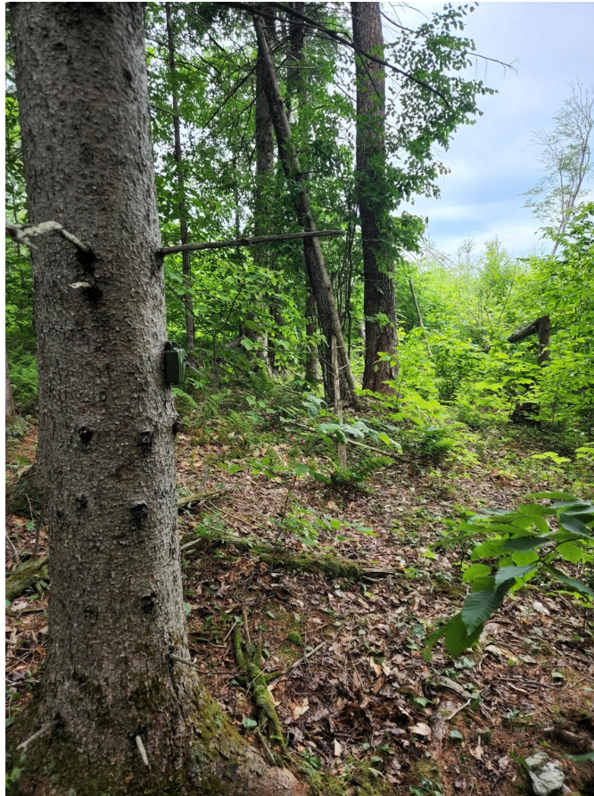
Figure 2: An example monitoring site in GMNF near a recent cut. Note the Song Meter Micro attached to the tree.
