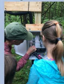
Alix Contosta (UNH) demonstrating sensor wiring to Vermont Commons School students while building a station on school woodlands in Charlotte, VT.
