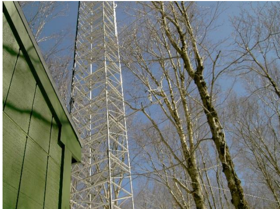
The FEMC takes meteorological measurements at 0.5, 7.5, 17, and 24 meters above the forest floor at 1300' at the canopy research tower at the Proctor Maple Research Center in Underhill, VT.
