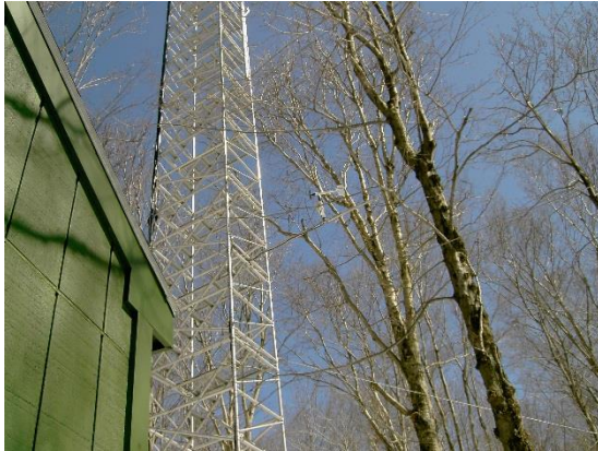
The VMC takes meteorological measurements at 0.5, 7.5, 17, and 24 meters above the forest floor at 1300' at the canopy research tower at the Proctor Maple Research Center in Underhill, VT.
