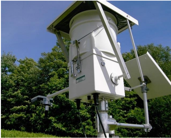
Automated Precipitation Collector at the VMC Air Quality Site in Underhill. Sampling at this site started in 1984.
