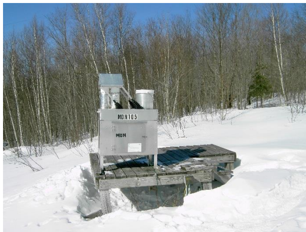
Aerochemetrics (ACM) collector for capture and analysis of mercury contained in precipitation.
