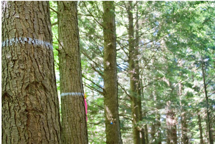
Figure 8. In locations where permitted, trees that land within the FHM plots are painted to mark the location that DBH was measured to ensure consistency from year to year.
