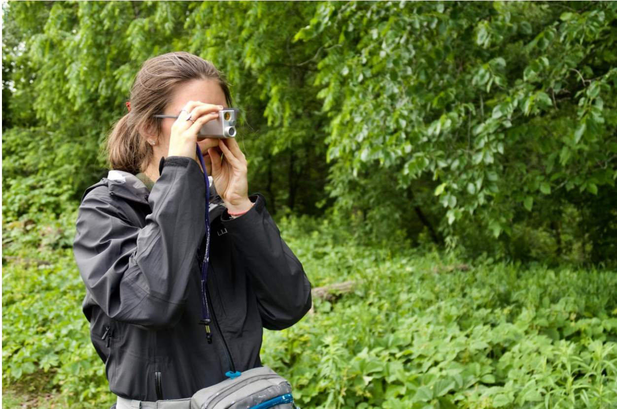
Figure 9. Measuring height with a Haglof hypsometer.
