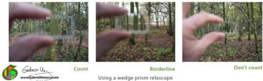
Figure 22. Examples of using a wedge prism. Photos courtesy of Gabriel Hemery, at www.GabrielHemery.com .
