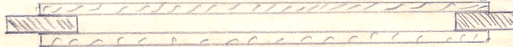
Fig. 1. Showing the iron bars and blocks that form the closed magnetic circuit of the Double-Bar Permeameter.
