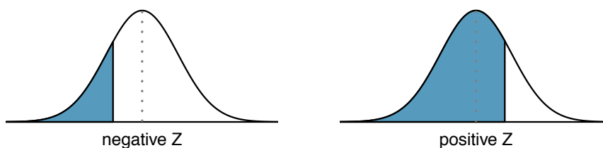
Figure 3.7: The area to the left of Z represents the percentile of the observation.
