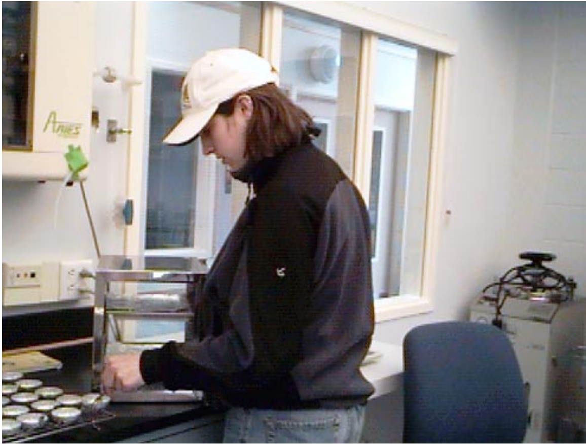
Figure 8: Marianne, placing weighed, dried samples on the oven tray for transfer to the furnace.
