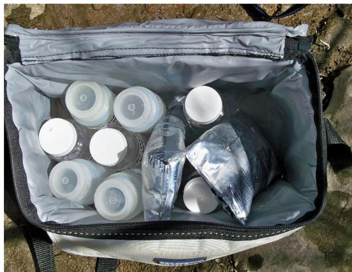
*Figure 9: Cooler for Transporting Samples back from field sites*
