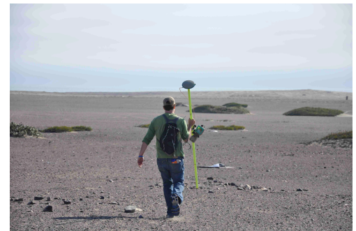
Dr. VanValkenburgh laying down ground control points for an Unmanned Aerial Vehicle flight using an RTK GPS system.
