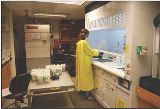
Quartz purification laboratory with dedicated polypropylene hood for acid transfer and 10 ultrasonicators for sample treatment.
