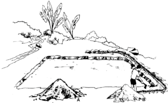
Figure 11: Digging a 'core trench' (A= Topsoil, B= Clay)
